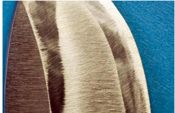
Section of a hard hollow ground blade sharpened as described in the last paragraph.
