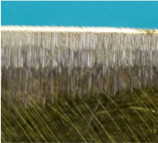
Enlargement of a soft blade, showing file marks & steeled edge at the top.
